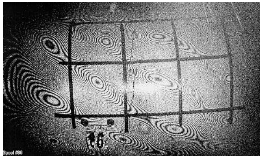
Figure 4. Spool section showing strong spiral wave.
